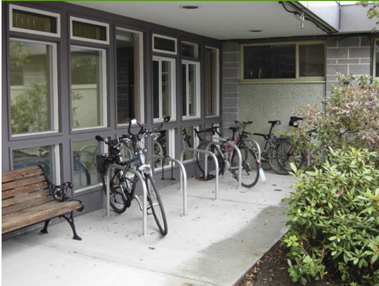
To help deter theft, weather-protected bicycle racks were set up in places where they could be seen from the inside of Saanich's municipal buildings (Photo: District of Saanich).
