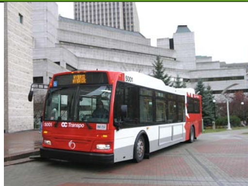
One of Ottawa's two hybrid diesel-electric buses. Photo courtesy of OC Transpo.
