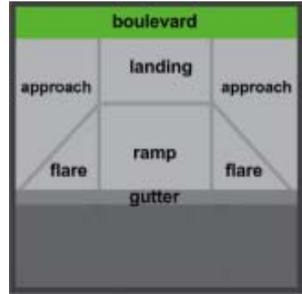
Figure 3–6: Curb Ramp Components
