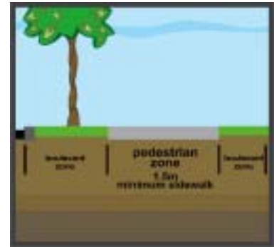
Figure 3–1: Pedestrian Zone in Typical Residential Street
