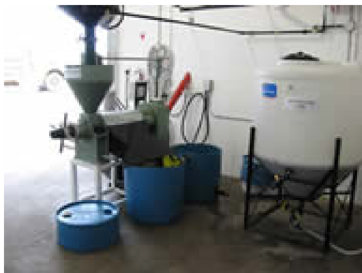
Seed press and oil storage for biodiesel production at the Olds College BioFuel Technology Centre (Photo: OCSI/ Carien Vandenberg)
